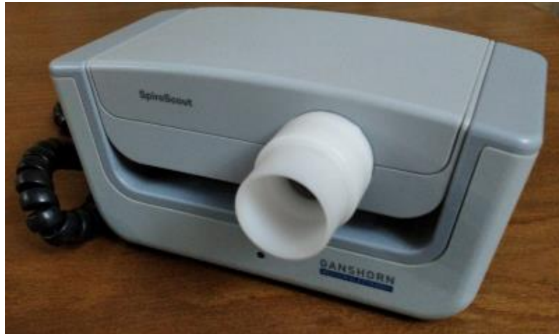
Figure 2. Ganshorn Medizin Electronic GmbH spirometer made in Germany to examine the results of spirometry flow-volume measurements and indices
