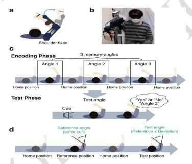
a. Setup and experimental tasks for measuring proprioceptive function of participants
